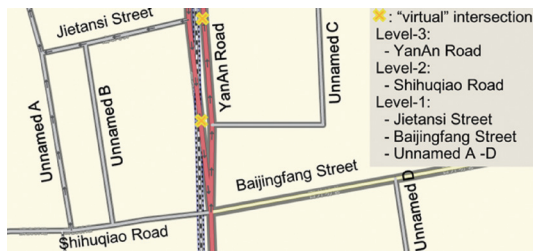
Fig. 1. Road network pre-processing with “virtual” intersections and level-of-road annotations
