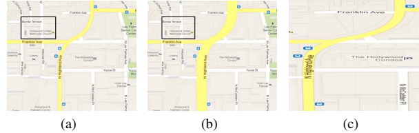
Figure 3: Comparison of our algorithm with linear zooming. (a) A map with a road and a region of interest highlighted in the black rectangle. (b) The result after broadening the road by 50 pixels. (c) The result after linearly enlarging the whole image by 300%.
