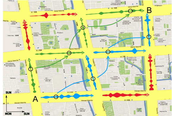
Figure 7: Time series curves representing the time consumed by taxis on each road segment of one Friday in one-way direction from location A to B. Different time saving routes could be found out at different times in a day.
